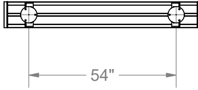
1119-06-M3 FOOTING SPACING
