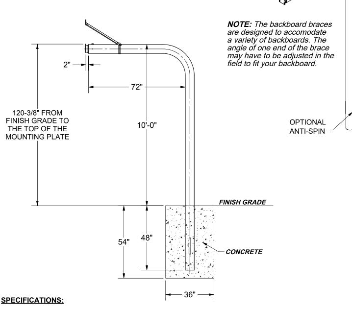
**Material:** Support post is a single length of 6-5/8" O.D. galvanized steel formed to provide a graceful 6 ft. offset. Backboard mount is a 6-1/4" x 6-1/2" steel plate welded to the sleeve adapter then mounted to the support post with a set screw and drive pins.
