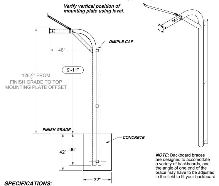
**Material:** Support post is a single length of 4-1/2" O.D. galvanized steel formed to provide a graceful 4 ft offset. Provided as an extra vertical stabilizer, the Truss Post Brace running parrellel of goosenceck post is a 3-1/2" O.D. galvanized steel tube connected by welding two stubs perpendicular. Backboard mount is a 6-1/4" x 6-1/2" schedule 40 steel plate welded to the GNP sleeve adapter then mounted to
