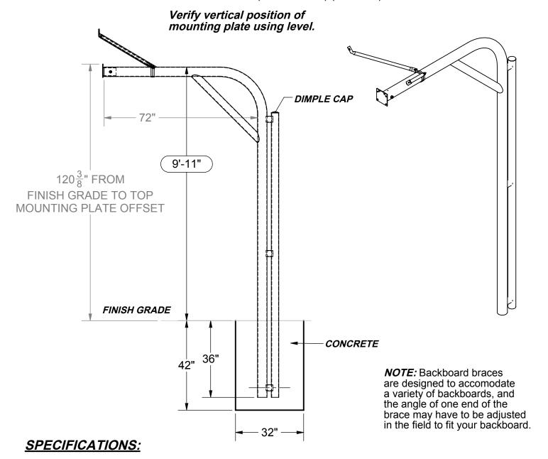
**Material:** Support post is a single length of 4-1/2" O.D. galvanized steel formed to provide a graceful 6 ft offset. Provided as an extra vertical stabilizer, the Truss Post Brace running parrellel of goosenceck post is a 2 3/8" O.D. galvanized steel tube connected by welding two stubs perpendicular. Backboard mount is a 6-1/4" x 6-1/2" schedule 40 steel plate welded to the GNP sleeve adapter then mounted to
