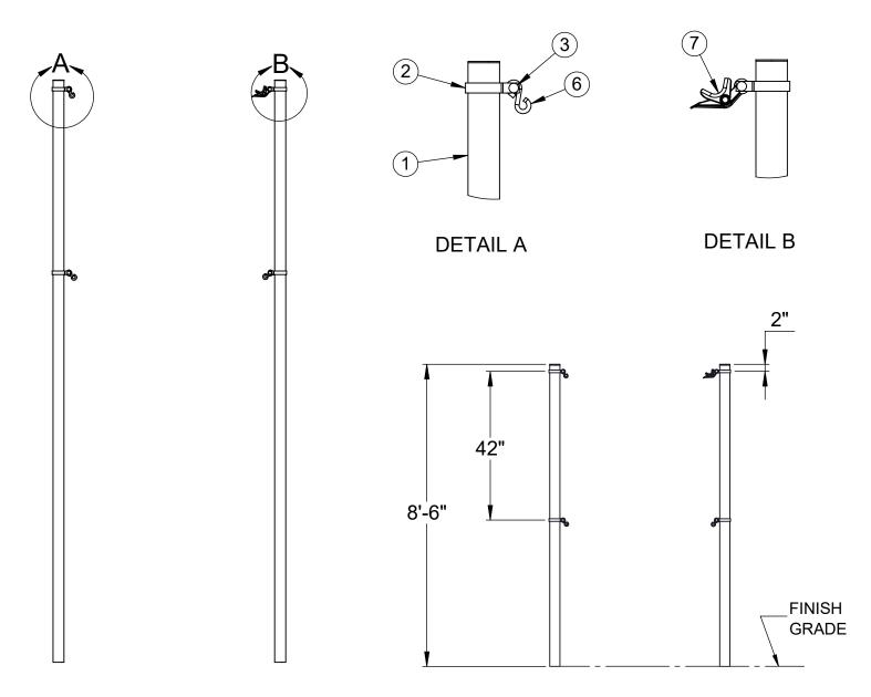
INSTALL THE POSTS IN  $\emptyset$  18" x 24" DEEP CONCRETE FOOTINGS OR POST SLEEVES. THE TOPS OF THE POSTS ARE 8'-6" ABOVE THE FINISH GRADE.
