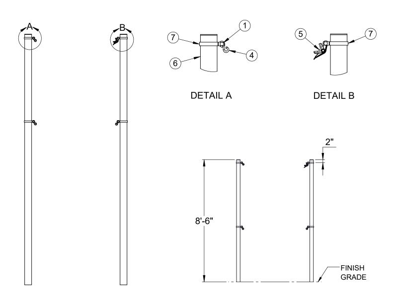
INSTALL THE POSTS IN  $\phi$  18" x 24" DEEP CONCRETE FOOTINGS OR POST SLEEVES. THE TOPS OF THE POSTS ARE 8'-6" ABOVE THE FINISH GRADE.
