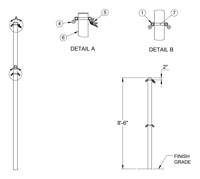
INSTALL THE POST IN A  $\phi$  18" x 24" DEEP CONCRETE FOOTING OR POST SLEEVE. THE TOP OF THE POST IS 8'-6" ABOVE THE FINISH GRADE.
