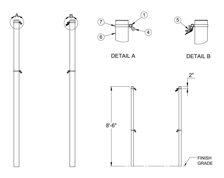
INSTALL THE POSTS IN  $\phi$  18" x 24" DEEP CONCRETE FOOTINGS OR POST SLEEVES. THE TOP OF THE POSTS ARE 8'-6" ABOVE THE FINISH GRADE.
