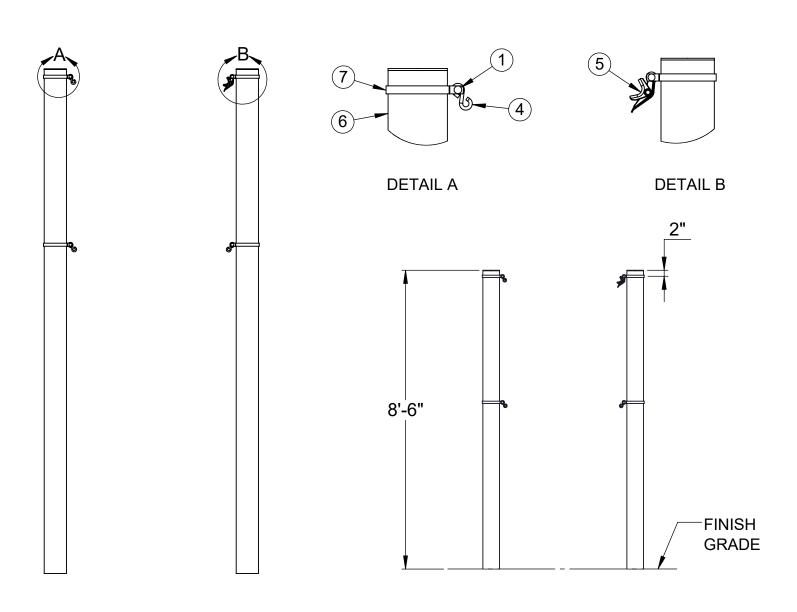
INSTALL THE POSTS IN  $\oslash$  18" x 24" DEEP CONCRETE FOOTINGS OR POST SLEEVES. THE TOPS OF THE POSTS ARE 8'-6" ABOVE THE FINISH GRADE.
