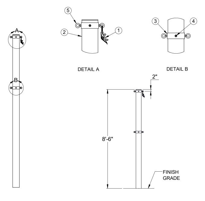
INSTALL THE POST IN A  $\phi$  18" x 24" DEEP CONCRETE FOOTING OR POST SLEEVE. THE TOP OF THE POST IS 8'-6" ABOVE THE FINISH GRADE.
