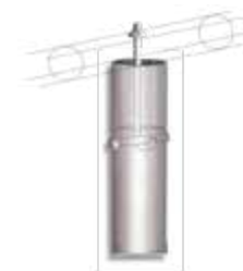
MODEL #8346-30 J-Hook Illustration Inside of sleeve
